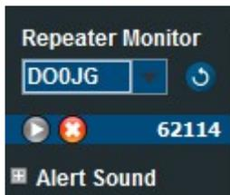
In the Drop Down menu you can select the repeater you want to monitor. Before you can use this option you have to set up your repeater in the setting (will be explained later in this manual)
